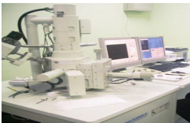
Figure 5: Photos of SEM & EDX
