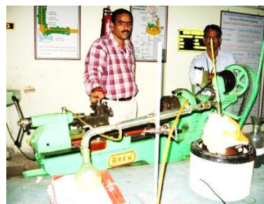
Figure 1, Experimental setup of fractional distillation to extract plastic petrol from liquid hydrocarbons
