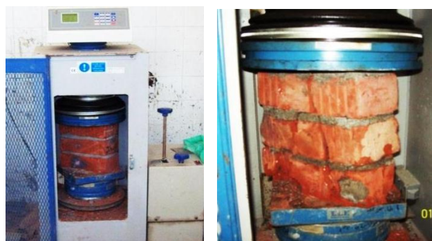
a. testing masonry prisms b. Failure of Prism
