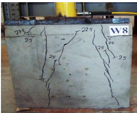
Figure 6 Crack Pattern of W8
