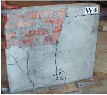
Figure 4 Crack Pattern of W4 with One Layer Interface
