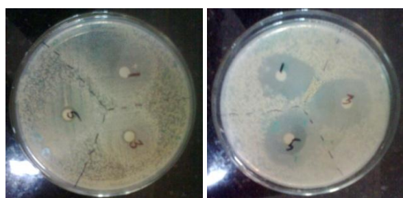
(A) (B) Fig.11 : (A) - E.coli treated with 1mM, 3mM and 5mM (A) AgNO 3 discs( 1mM, 3mM and 5mM), (B) - E.coli with Ag nanoparticles discs( 1mM, 3mM and 5mM)
