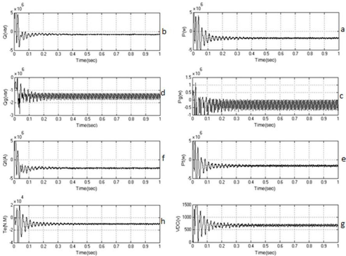
**Figure (9):** output power of the simulated system for machine speed of 2160 RPM at voltage imbalance mode: a) active power of stator , b) reactive power of stator , c) active power of the converter located on network side , d) reactive power of the converter located on network side , e) active power of infinite bus , f) reactive power of the converter located on network side , g) DC link voltage , h) Electromagnetic Torque
