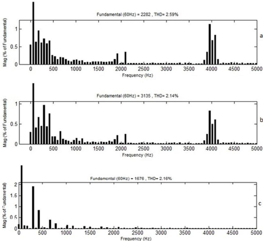
**Figure (4):** Output current of the simulated system for machine speed of 2160 RPM at voltage balance mode : a) THD of stator current, b) THD of infinite bus current , c)THD of injecting current from the converter located on network side
