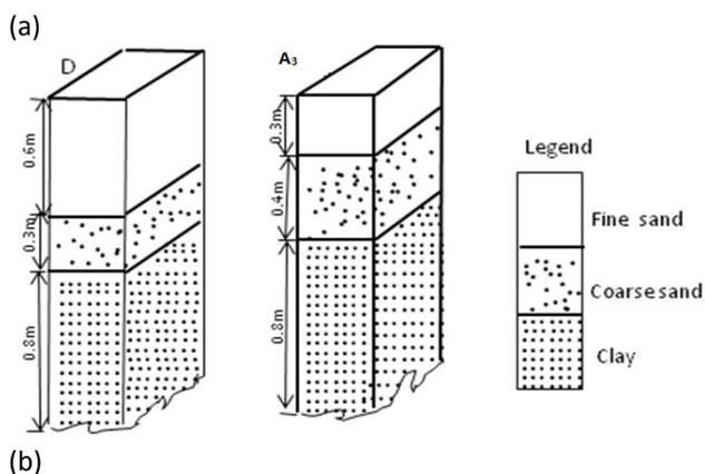
**Figure 6:** Field data pseudosection, theoretical pseudosection and ERT of Traverse 3; (c.) Soil profile in pits D and A<sub>3</sub>, on Traverse 3, Odo-Oba Flood plain, South-western Nigeria
