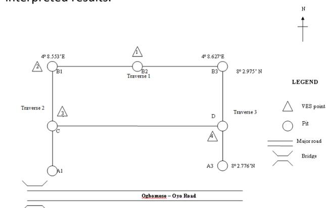
**Figure 3:** Outlines of profiles, pits and Vertical Electrical Sounding points in the study area.
