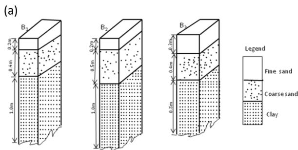
**Figure 4:** (a.) Field data pseudosection, theoretical pseudosection and ERT of Traverse 1; (b) Soil Profile in pits B<sub>1</sub>, B<sub>2</sub> and B<sub>3</sub> on Traverse 1, Odo-Oba Flood plain, South-western Nigeria
