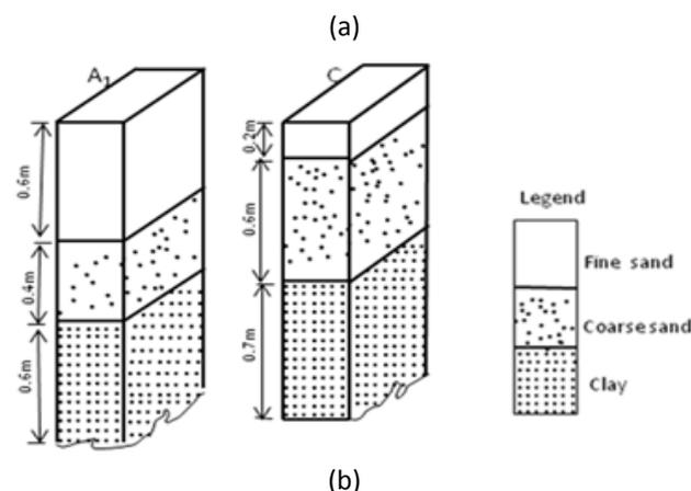
**Figure 5:** Field data pseudosection, theoretical pseudosection and ERT of Traverse 2; (b) Soil profile in pits C and A<sub>1</sub>, on Traverse 2, Odo-Oba Flood plain, South-western Nigeria
