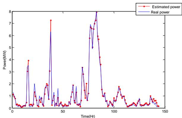
**Figure 6** Wind power prediction for the next one day in chester unit by Levenberg-marquardt algorithm
