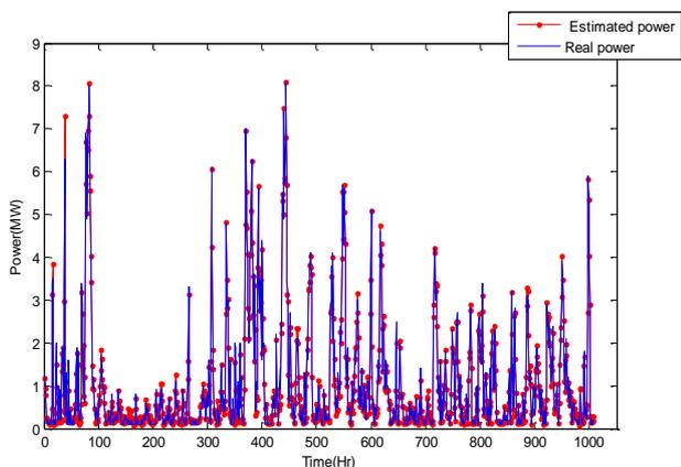
**Figure 11** Wind power prediction for the next seven days in chester unit by Pso algorithm
