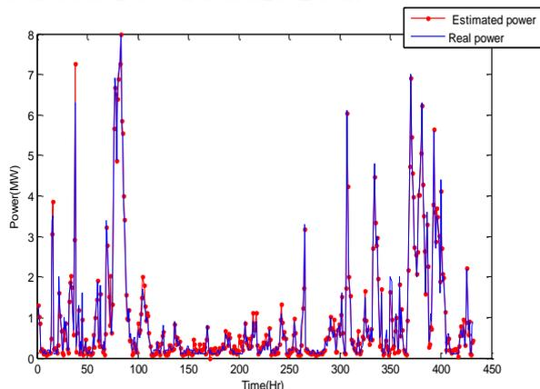
**Figure 7** Wind power prediction for the next three days in chester unit by Pso algorithm
