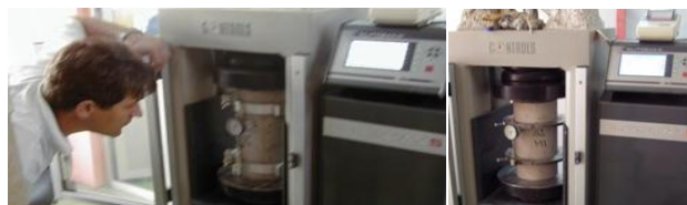
Fig. 4 Testing of Modulus of elasticity
