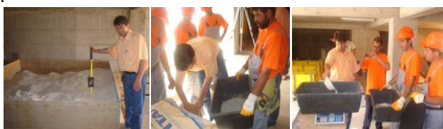
Fig.2 Measurement of the integral components of concrete
