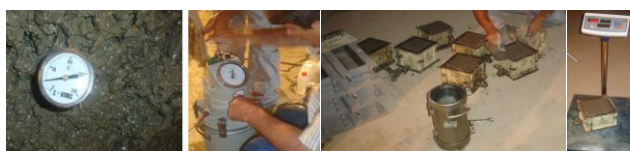
Fig. 3 Measuring the temperature and porosity on concrete
