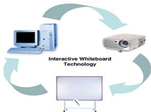
Fig1. By using video projection information can be seen and all applications on the computer can be controlled via touching the board, either with your finger, or with an electronic pen/stylus
