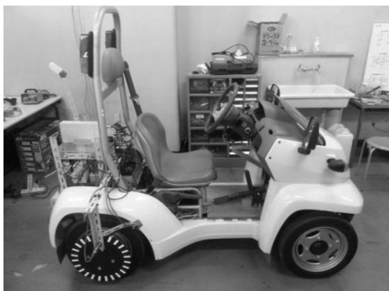
Fig.4 Analysis vehicle model of Toyota COMS
