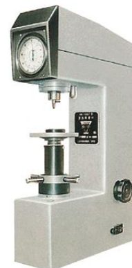
Figure 4: Rockwell Hardness Test Apparatus
