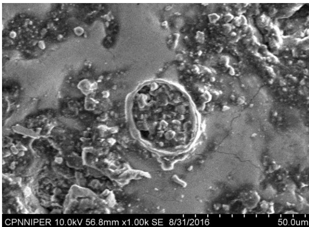
Fig.7 EN 31 stainless steel after Machining
