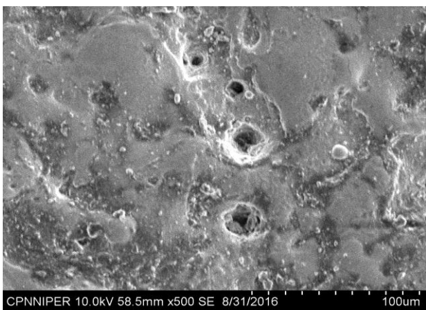
Fig. 6 EN 31 stainless steel after Machining
