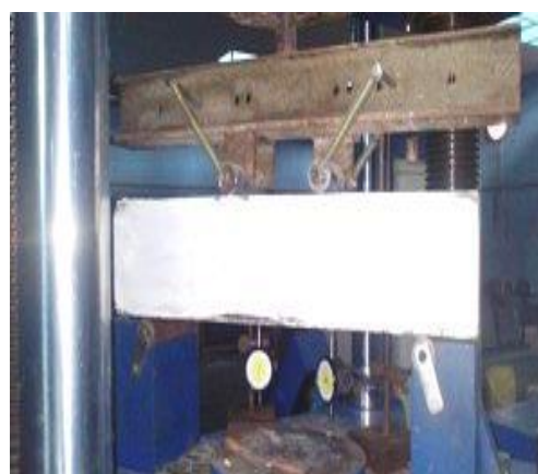
Figure 4: Experimental test set up of flexural loading
