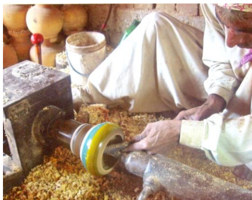
Plate.11 Lac-turnery on electrical lathe.
