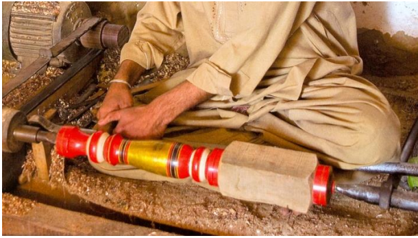
Plate.5 Electric Lathe ( jandrī )
