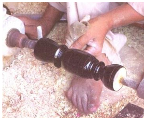
Plate.13 Last coat of coloured lac, colour application from light to dark.
