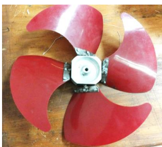
Figure 2.2 Variable blade angle propeller model (F)
