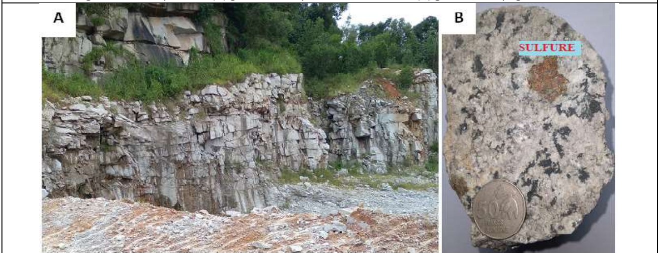
Figure 4: (A) Macroscopic appearance of SOMIAG quarry granites, (B) Inclusion of sulphide in a granite sample from the SOMIAG quarry
