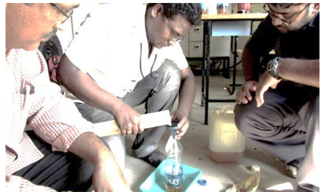
Figure 5, Blending of Plastic Petrol with Gasoline (50%+50%)
