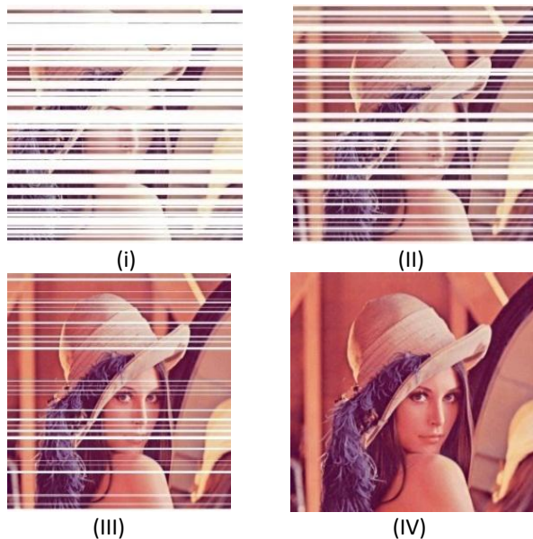
Fig.4. Reconstructed image after receiving pairs of column concurrently, PSNR values (i) 25.2837dB (ii)26.5822 dB (iii) 30.6938dB (iv) Reconstructed image 40.71 dB[4]
