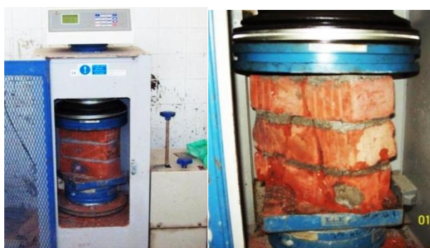
a. testing masonry prisms b. Failure of Prism
