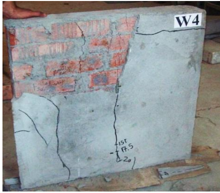
Figure 4 Crack Pattern of W4 with One Layer Interface
