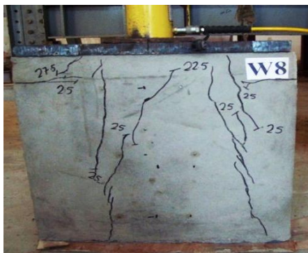
Figure 6 Crack Pattern of W8
