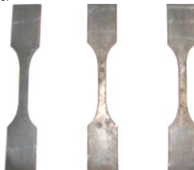
Fig 3- Carburization of low carbon steel samples
