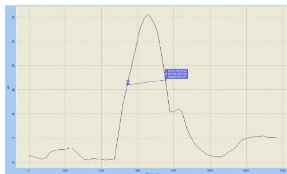
Fig. 8: Line profile of Ag nanoparticles obtained by 5mM AgNO 3 and Lemon extract
