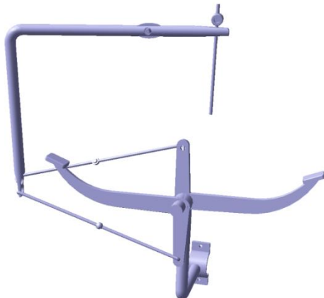
Fig.3 3D model – New clutch pedal
