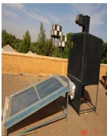
Fig. 1 Natural convective solar dryer
