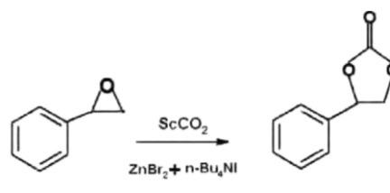
Fig.4. Reaction of styrene oxide with \text{CO}_2 to styrene carbonate in the presence of \text{scCO}_2
