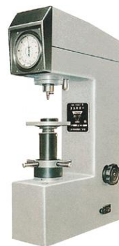
Figure 4 Rockwell Hardness Test Apparatus
