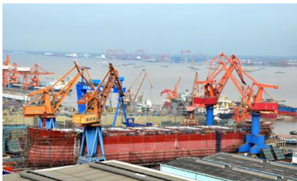
Fig. 3: Example of hull erecting
