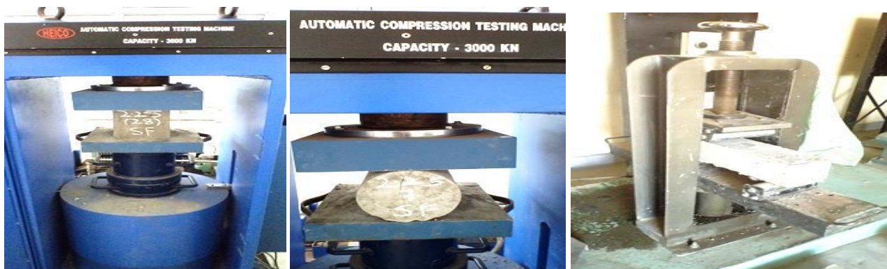
Figure: 1 (a) CTM for compression test, (b) CTM for split tensile strength test, (c) Flexural testing machine
